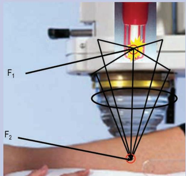
**Figure 3.** Focused shockwave with focal point (F<sub>1</sub>) in the sparkplug of the electrohydraulic generator and focal point (F<sub>2</sub>) at defined distance within the tissue. Positioning the opposing electrodes at the primary focus (F<sub>1</sub>) in a parabolic reflector results in a planar wave, which is emitted after the reflection of the primary spherical wave. The focal point (F<sub>2</sub>) of these plane waves is at an endless distance from F<sub>1</sub>.
