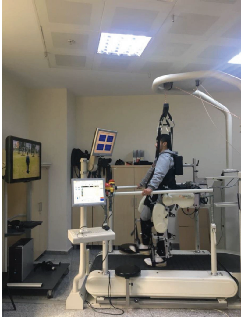
Figure 2. Lokomat, a robot-assisted gait training system.
