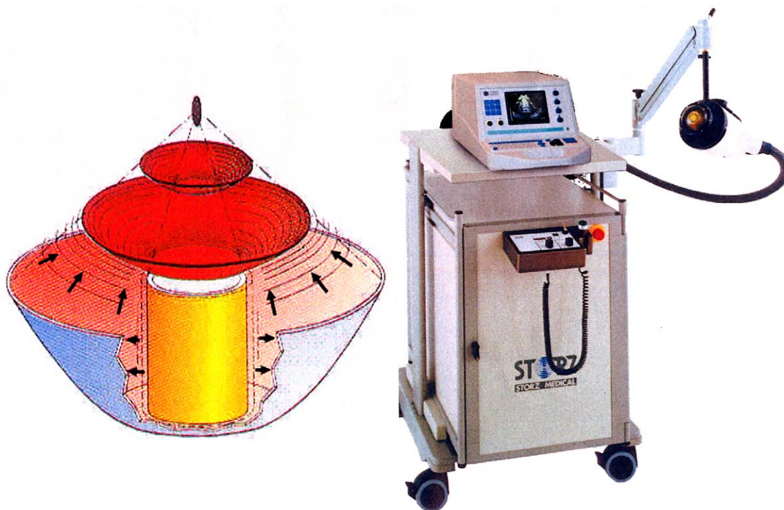
Fig 4. The electromagnetic generators have a mechanism similar to a loudspeaker. The electrical capacitor is discharged through a flat coil generating a rapidly changing magnetic field. This magnetic field induces an opposing magnetic field in a metal membrane above the coil, causing a repulsive force and rapid movement of the membrane. A special type of the electromagnetic transducer by one manufacturer uses a cylindrically shaped coil and membrane generating a radial movement of the membrane. The electromagnetic transducers are often referred to as EMSE systems (EMSE = electromagnetic shockwave emitter). When the coil moves outward, the pressure wave (arrows) is reflected to the focal point. The Storz Minilith with an inline ultrasound for focusing is shown. The generator head is on a flexible arm.
