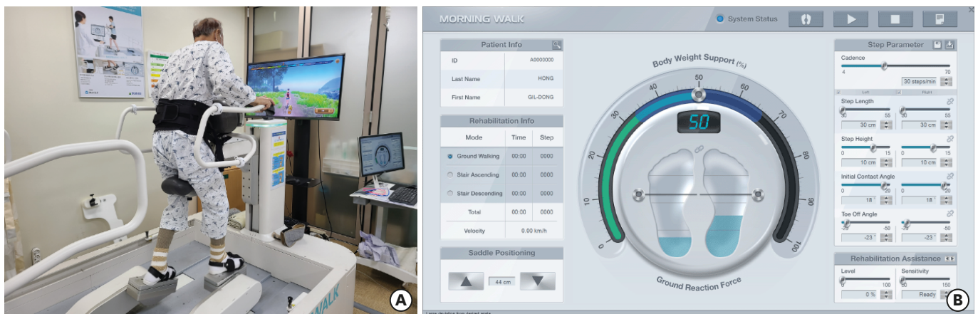
Fig. 1. (A) Morning Walk ® -assisted gait training with monitor-based virtual reality software. (B) Interface of Morning Walk ® for adjusting gait parameter and providing graphical information.
